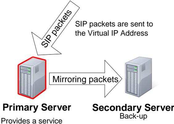
2. If the Primary server goes down, the Heartbeat feature switches the Secondary server to be the Primary server and assigns the Virtual IP address to the new Primary server.
